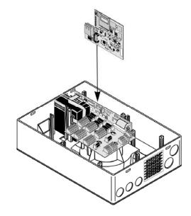
Figure 55: Installation of the TITANUS® network module
