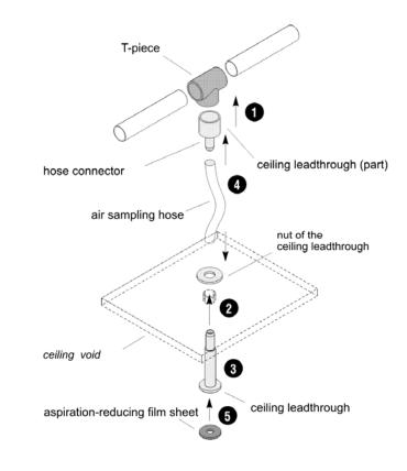
Figure 64: Installation of ceiling feed-through
