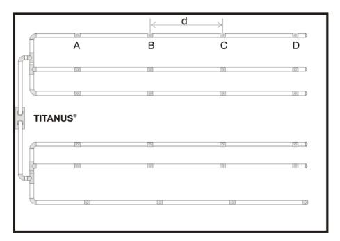
Figure 33: M-shape pipe system for area protection
