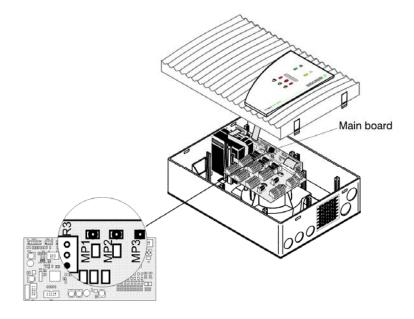
Figure 78: Adjustment dependent on the air pressure of the TITANUS® flow sensor
