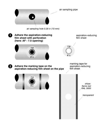
Figure 63: Attaching the aspiration-reducing film sheet
