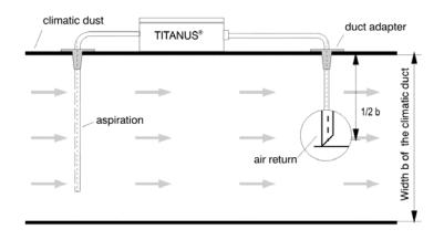
Figure 66: Positioning of air return in an air duct
