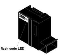
Figure 80: Position of flash code LED on the detector module
