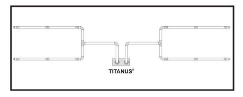
Figure 36: U-pipe system, e.g. for equipment protection
