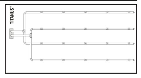
Figure 26: Pipe design for double knock detection
