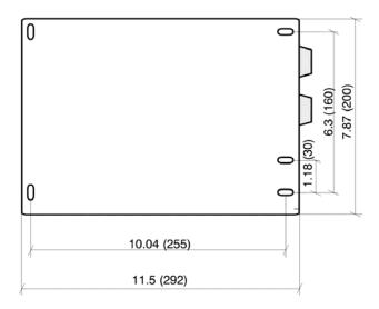
Figure 50: Borehole spaces of TITANUS® without support
