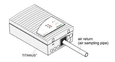
Figure 70: Mounting of the air return
