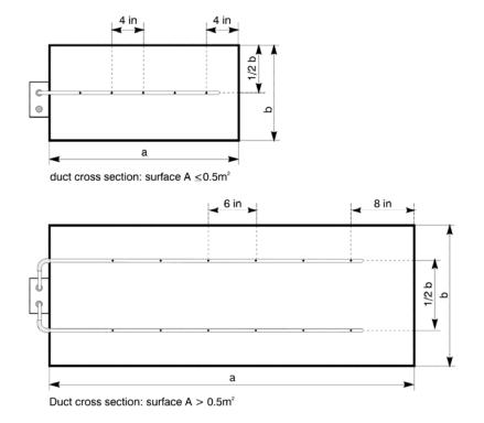
Figure 44: Ducts with small and large duct cross-section
