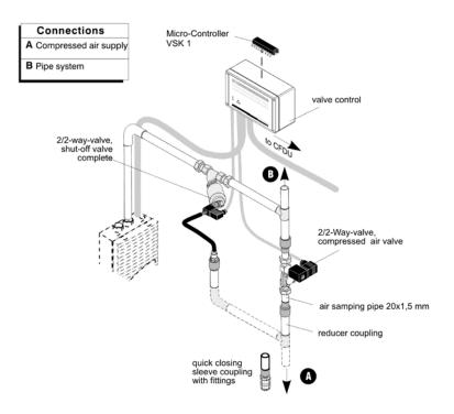
Figure 14: Components for automatic purging
