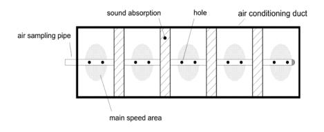
Figure 41: Sound suppressors in a duct
