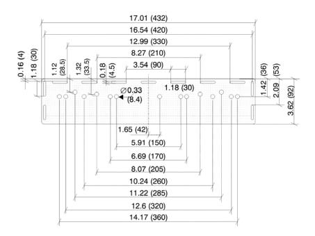
Figure 51: Borehole spaces of the support type MT-1
