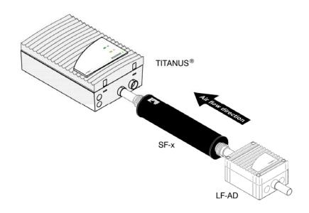
Figure 69: TITANUS® with special filter and LF-AD
