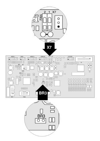
Figure 47: Changing fan voltage on the main board
