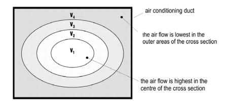
Figure 39: Rate distribution in an air conditioning duct with v1 > v2 > v3 > v4
