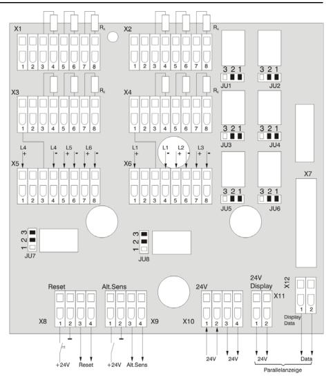
Figure 53: General layout of the circuit board terminal blocks
