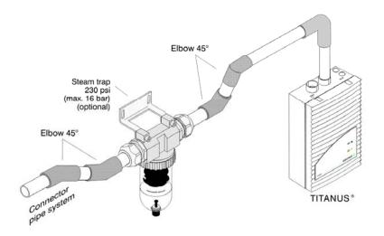
Figure 73: Installation of steam trap Type KA-DN-25 to pipe system
