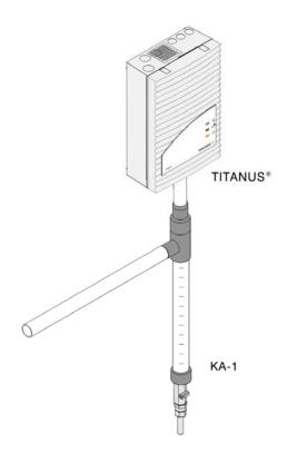
Figure 23: Type KA-1 steam trap to eliminate water vapor from the pipe system and to collect the condensate from the pipe system
