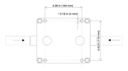
Figure 67: Spacing for bore holes on base of air filter housing
