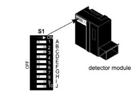
Figure 46: Default settings on the TITANUS® detector module
