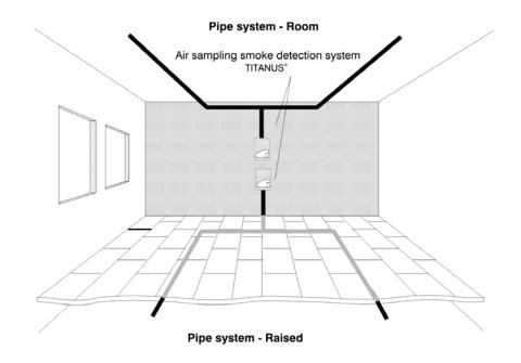
Figure 1: Principle of room monitoring with the TITANUS<sup>®</sup> air sampling smoke detection system
