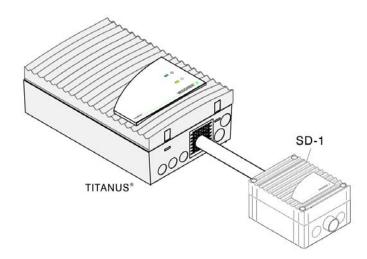
Figure 71: Mounting of noise suppressor
