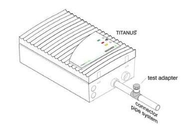
Figure 75: Mounting of the test adapter at the pipe system
