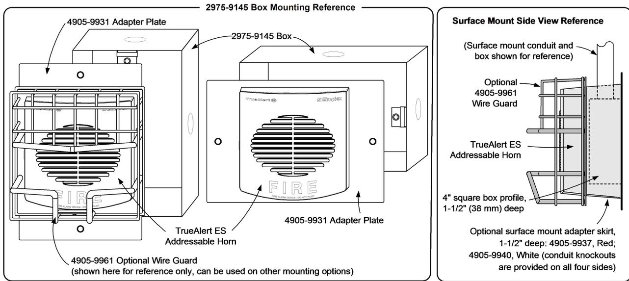
**Figure 3: Adapter Plate and Surface Mount Installation Reference**
