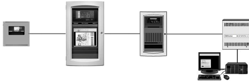
Figure 6: Single run linear network topology (no T-tapping)
