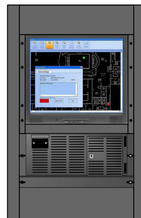
Figure 5: Rackmount PC and Monitor
