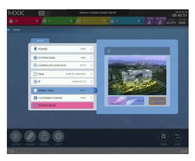
Touching the aerial view button on the setting screen displays the screen above. The aerial view is the image that appears on the initial screen of the panel.
