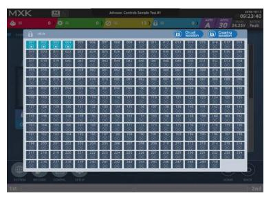
Devices connected to the loop are colored in blue, and devices not connected are in black.
