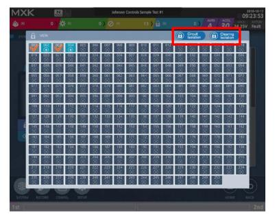
The selected devices have a check mark ( $\checkmark$ ), and Touching the Circuit Isolation or Clearing Isolation button in the red square. When you select Circuit Isolation, the following screen appears:
