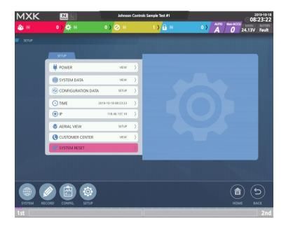
The screen that appears when you touch on the Setup menu in the initial screen provides data to be set or changed on the panel.
