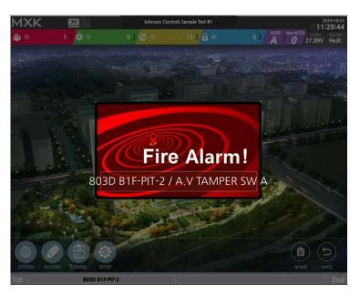
The screen appears when a fire occurs on the initial screen. The bottom of the screen displays information about the  $1^{st}$  fire and  $2^{nd}$  fire.
