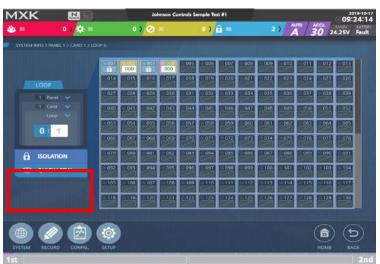
There are too many I/O modules to be displayed on the screen. In order to see the states of all the I/O modules, the system supports a screen as below.
