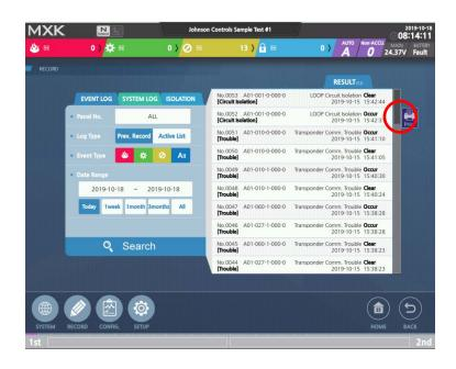
In order to print out records, touching the Print button on the upper right corner of the screen displays the following screen.
