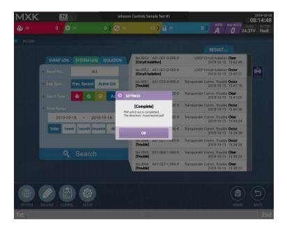
When the file saving is completed, the screen above will be displayed. The path appears with the completion message.
