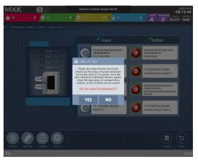
The screen above describes the hazards that may occur during the output test, and the user must read it before the test and pay a special attention to the damage that may result from the test.
