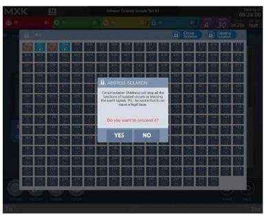
Once the circuit isolation is completed, you can check the state of circuit isolated I/O modules.
