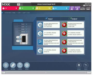
This screen appears when you touch on a device (I/O module's icon) on the loop information screen. This is the status of MXK44 I/O module. The screen shows the type of input device and the output device connected to the I/O module along with the status of the input device's end-of-resistor and the zone (the area where the input and output devices are connected).
