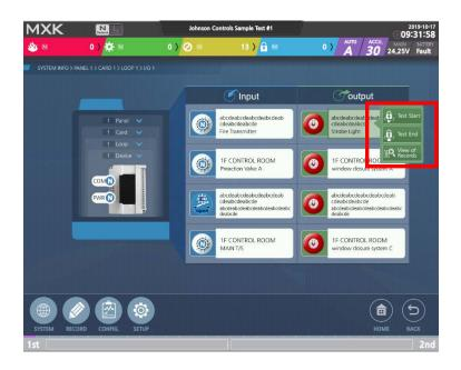
If you want to perform a forced test on the output, Touch the green square boxes on the screen above which represents the output zone on the screen of I/O module state, and the Touched icon will be inverted as shown in the screen above. In this state, Touch the circuit test in the submenu and you are ready to test the output.
