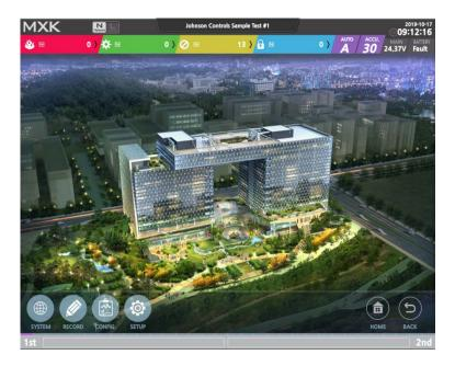
This is the initial screen that is displayed at the end of the initializing screen. Touching the area of the number of events at the top of the screen shows up to 10 latest records of corresponding events. Auto-Restoration/Latched mode is displayed on the right side of the event area and the mode can be changed by touching the mode area.
