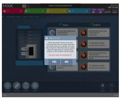
This screen appears when you touch the circuit test button in the previous screen. It explains the hazards that may occur during a circuit test. Before the test, a user should read it and pay special attention to the enormous damage that may be caused by the test.
