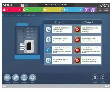
This screen appears to show the state of MXK22 I/O module when you touch a device (the icon of I/O module) on the loop information screen.
