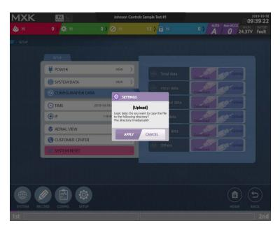
This screen appears when you Touch Download/Upload from the previous screen. The guide message will be displayed and you can touch on the Apply button to actually apply the data to the system, or Touch the Cancel button to remove the message.
