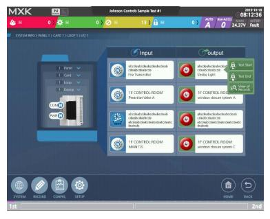
If you want to perform a forced output test, Touch on the square box (where reads the "Strobe Light"). Touching the circuit test in the submenu is ready to test the output.
