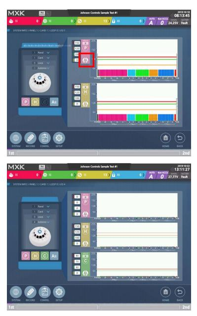
The screen above is about an analog type detector with two or three kinds of information. Touch the red box of the screen to see the warning statement and to isolate the circuit.
