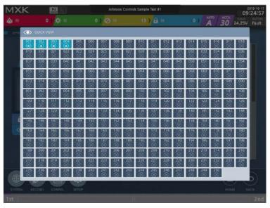
The screen helps you to check the status of all devices connected to the loop.
