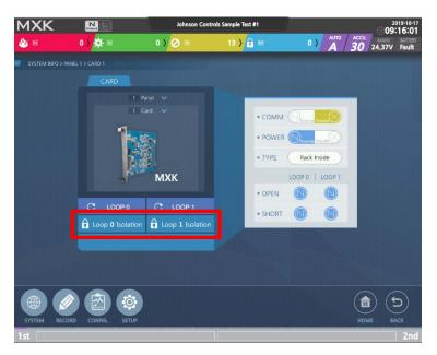
The buttons in the red square are used to isolate circuits by loop. Touch Loop 0 isolation and see a warning message as shown below.
