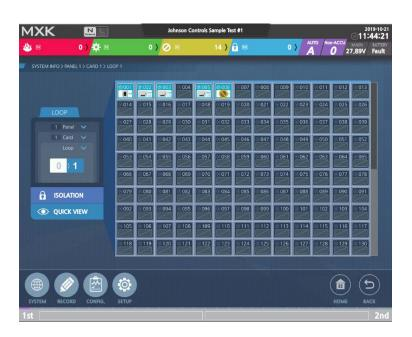
The screen above is shown when a loop has a trouble, indicating that there is a trouble with No. 6 I/O module on the Loop 0 in No.1 transponder.
