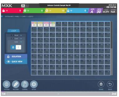
Touching the icons of LOOP 0 and LOOP 1 on the card (Transponder) Statue view shows the screen above. The current screen shows the type and status of devices connected to LOOP1 of 01 transponder.
