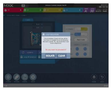
Touching Isolate will block the loop 0 and the square of the Loop 0 changes to have a yellow rim on the next screen.
