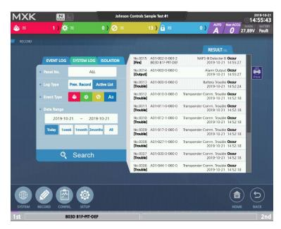
This screen shows a currently active list for an area where fire occurs. This screen appears when you touch the Record icon on the bottom of the screen. Select the currently active list in the search fields and Touch Search to see the corresponding area and the type of activated detectors. The 1<sup>st</sup> Fire and 2<sup>nd</sup> Fire keep being displayed in any screen of any menu until the fire is restored to normal and the fire indicator icon keeps being displayed.
