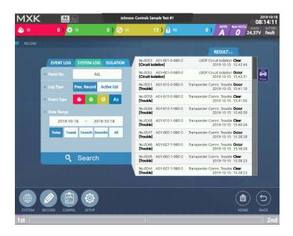
This screen shows the past records of fire and the area where fire occurred and it appears when you touch the Record icon on the bottom of the screen.
