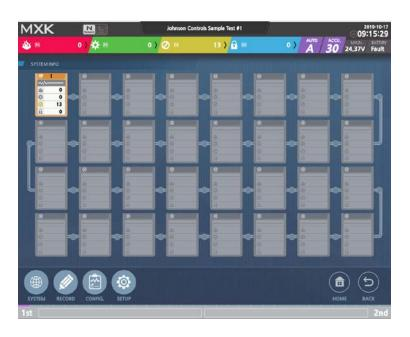
This screen appears when you touch on the system menu. It displays the state of each panel connected to the network as above. You can see the number of events on each corresponding panel.
