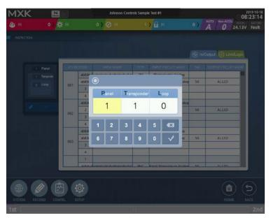
The screen above is to select a location to confirm the corresponding input & output. A user can select a panel, a transponder, and a loop.
