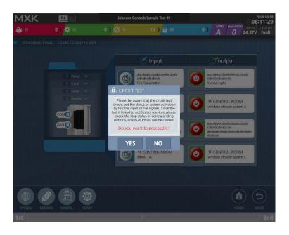
The pop-up window describes the hazards that may occur during the output test, and the user must read it before the test and pay attention to enormous damage that may result from the test.
