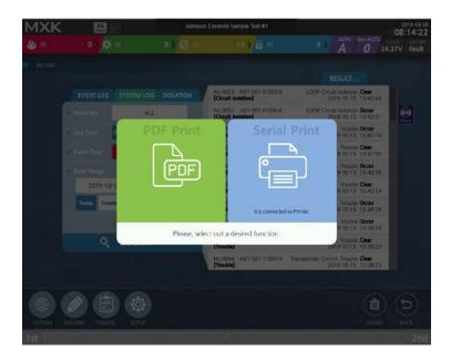
Select the Serial Print. If it is not selectable, make sure that the print connection is OK.
