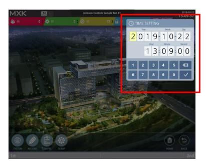
Touching the time area at the right side of the initial screen presents a sub menu to set a time as above. If you set the time, all of the panels on a network have its time synchronized with your panel.
