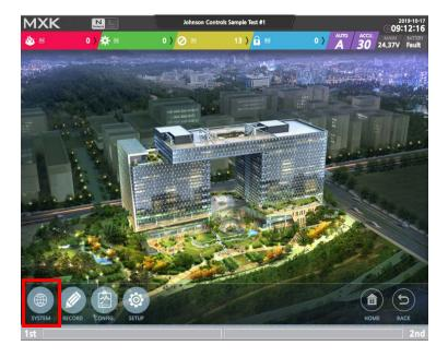
Touching the system menu at the bottom of the screen, a screen on the next page will appear: This menu allows you to check the states of the panels linked to the system, the transponders connected to the panels, and the I/O modules connected to the transponders. You can check the current states like faults, fires, etc. and go to the menu to conduct forced input/output tests.
