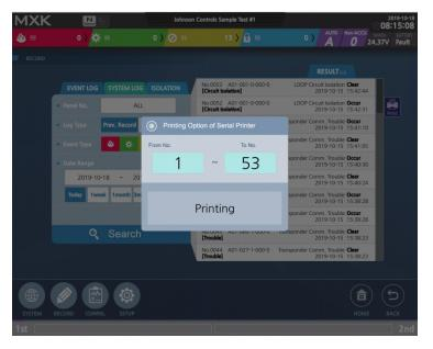
When the Printing button is activated, the range values are fixed and cannot be changed; if you want to make changes, Touch another area to start from the beginning. Once the desired range is selected, select the Print button. Upon selected, the print-out will proceed as shown in the screen below.
