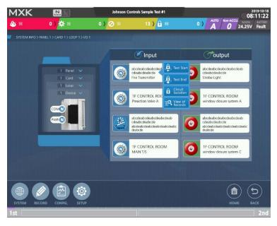
An inverted image in the Input or Output area means that this circuit is selected.
