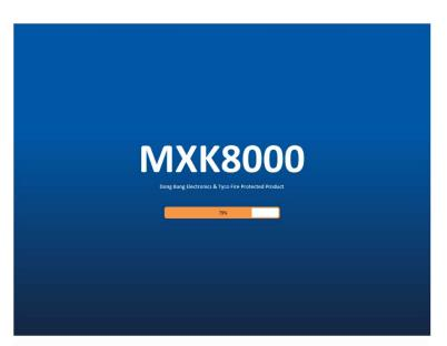
This screen shows the process of initializing the system after the initial power is applied to the panel. Before booting, if USB is connected to the MCM board, the system is automatically updated with files in the specified directory (top:₩mxk8000). As the updates finishes, the booting starts.
