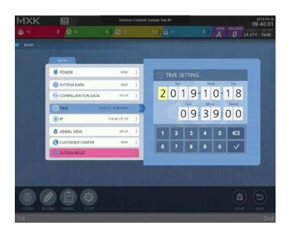
Touch the Time button on the setting screen to display the screen above. Time plays an important role because it represents the time displayed in the upper right corner of the screen and is one of criteria used to record events occurring from the device or system.
