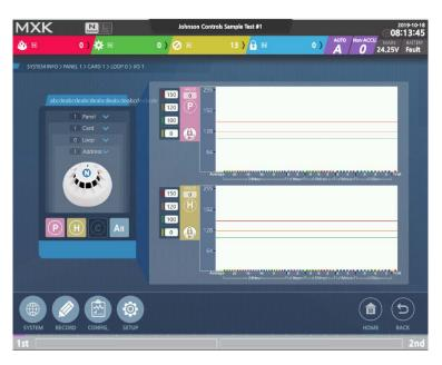
The screen above is about an analog detector with a maximum value of 127. On the left side of the screen, analog information of P (optical), H (quantitative), and C (carbon monoxide) types can be checked, and non-applicable type is disabled and cannot be read. On the right side of the screen, the reference level and the level values received from the detector are recorded in a graph.
