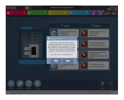
The screen appears when you touch the circuit test button on the previous screen. The window describes the hazards that may occur during a circuit test. Before the test, a user should pay special attention to the enormous damage that may be caused by the test.
