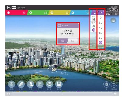
**Touching** the **Auto-Restoration/Latched mode** area opens a sub-area on the left where you can configure the mode. Select either **Auto-Restoration** or **Latched mode**, then touch the lower setting button. A confirmation pop-up window will appear. Touch **Apply** to finalize the mode setting.
