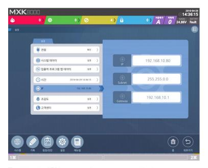
Touching the 'IP' button on the setup screen displays the screen above. This screen displays the IP information configured on the panel. This IP information is used for data exchange with workstations or other panels. Additionally, the subnet and gateway information are also displayed."
