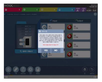
The screen above explains the hazards that may occur during the output test. The user must read this carefully before proceeding and pay special attention to the potential damage that could result from the test.
