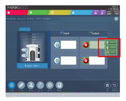
To perform a forced test on the output, touch the **green square boxes** on the screen that represent the output zone in the I/O module state screen. The touched icon will invert, as shown in the image above.
