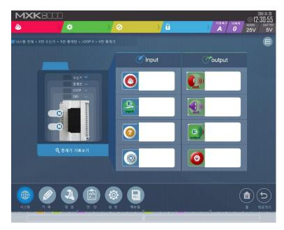
Navigating to 'Main Menu' > 'Panel State' > 'System' > 'I/O' displays this screen. If a detector connected to the I/O module is activated by fire, the fire icon is displayed. The screen also shows the operational status of the output equipment connected based on the I/O map.
