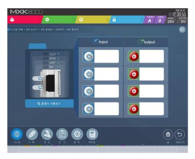
This screen appears when you touch a device (I/O module's icon) on the **Loop Information Screen**. It shows the status of the **MXK44 I/O module**.
