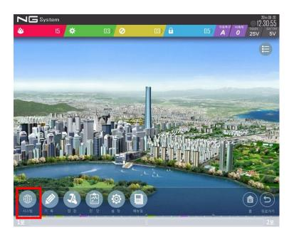
Selecting the **system menu** at the bottom of the screen opens the next page. This menu allows you to check the status of panels linked to the system, the transponders connected to these panels, and the I/O modules connected to the transponders, view the current states, such as faults and fires and access a menu to perform forced input/output tests.
