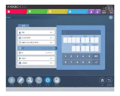
Touching the 'Time' button on the Setup screen displays the screen above. Time is crucial as it is displayed in the upper right corner of the screen and used to record events occurring within the device or system. The current time is displayed, and any changes made to the time are applied to the system immediately.
