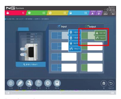
To perform a forced output test, touch the square icon representing the output zone (as shown in the screen above, labeled "Experiment Building 1, 4th Floor, Local Alarm") in the Relay Status Screen. The touched icon will invert, as shown in the image above. Once this is done, touch Circuit Test in the submenu to complete the output test preparation.
