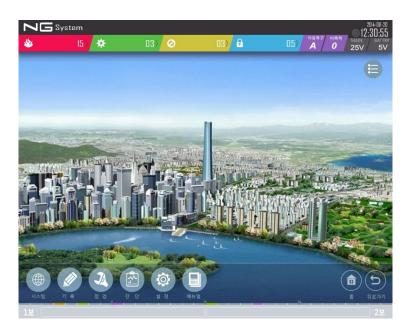
This is the initial screen that is displayed at the end of the initializing screen. Touching the number of events at the top shows up to 10 of the latest records. The right side of the event area displays 'Auto-Restoration' or 'Latched mode,' which can be toggled by touching the mode area.
