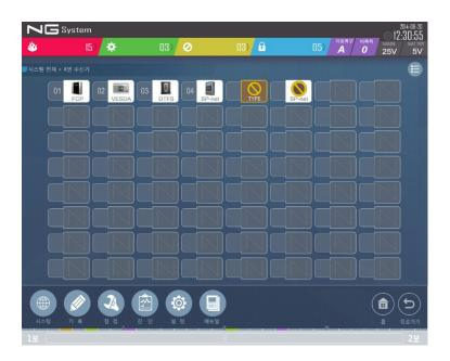
This screen appears when you touch Detailed View in the sub menu of each panel image on the screen on the previous page. It displays the status of the transponder connected to the panel as shown above.
