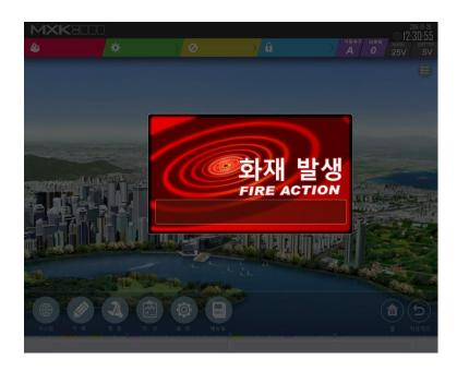
This screen appears when a fire occurs on the initial screen. The bottom of the screen displays information about the first and second fires.
