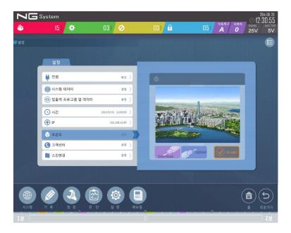
Touching the 'Aerial View' button on the setting screen displays the screen above. The aerial view refers to the image displayed on the initial screen of the panel. The screen allows you to download or upload screen images
