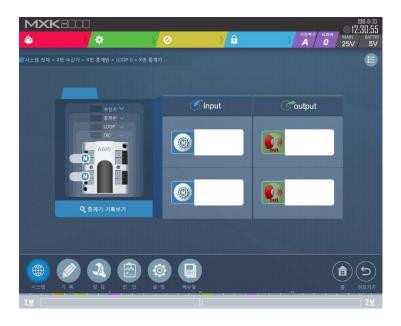
When you touch a device (I/O module icon) on the loop information screen, the MXK22 I/O module status screen appears.
