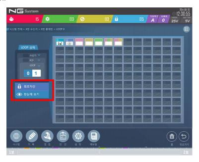
The system provides a **Quick View** feature for I/O modules, allowing you to monitor their statuses effectively, even when there are too many modules to display at once.
