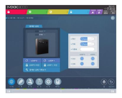
This screen appears when you select the image of a transponder in the Detailed View of the system. It displays the current status of the transponder, including communication, power, open status, shortage and redundancy.
