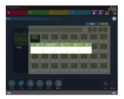
Touching the '+' button in the upper-left corner of the Inspection screen displays the screen above. This screen allows you to select a location for virtual input among a panel, a transponder, a loop, an address, and a point. Select the desired input, and the next screen will appear.
