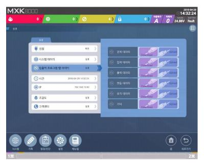
Touching the 'Configuration Data' button on the Setup screen displays the screen above. The 'In/Output Program and Data' button represents data used to control input/output links or activate fire/equipment. This data is collected from the site and transmitted to the panel using the input/output link table and site map within the Consys program.
