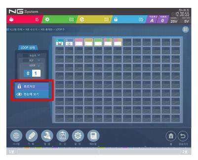
When you touch the Circuit Isolation button (located within the red square), a screen appears displaying the connected and disconnected devices in the loop.
