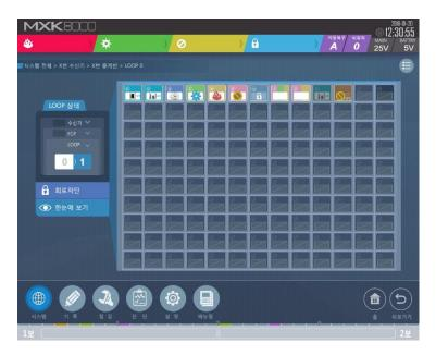
The screen above indicates a fault on Loop 0 of Transponder No.1, specifically with I/O module No.6. This screen does not provide the specific type of fault with the I/O module. To identify the exact type of the fault, touch the fault icon.
