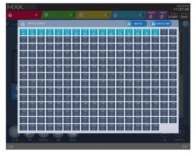
a screen appears displaying the connected and disconnected devices in the loop. **Connected devices** are highlighted in **blue** and **Disconnected devices** are displayed in **black** and are not
