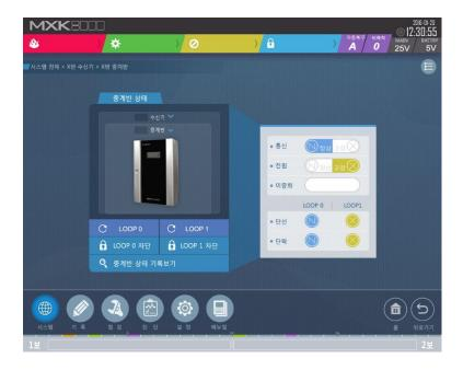
Touching a transponder to view its status displays the screen above. The right side of the screen shows information about communication troubles and power failures for the selected transponder. You can also view the fault states of Loop 0 and Loop 1, including open and short circuit statuses.
