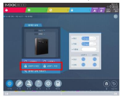
The buttons within the red square are used to isolate circuits by loop. Click Loop 0 Isolation, and a warning message will appear, as shown below.
