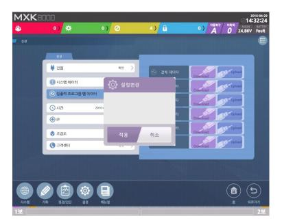
This screen appears after selecting 'Download' or 'Upload' on the previous screen. A guide message will be displayed. Click 'Apply' to apply the data to the system, or click 'Cancel' to dismiss the message.
