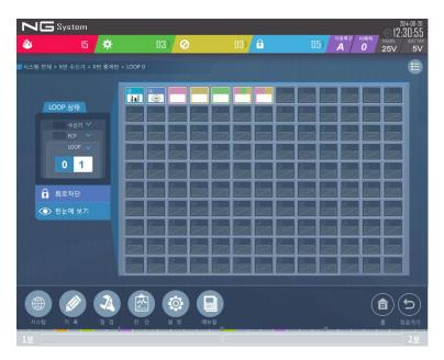
Touching the icons of LOOP 0 and LOOP 1 on the Transponder Statue view shows the screen above. The current screen shows the type and status of devices connected to LOOP1 of 01 transponder.
