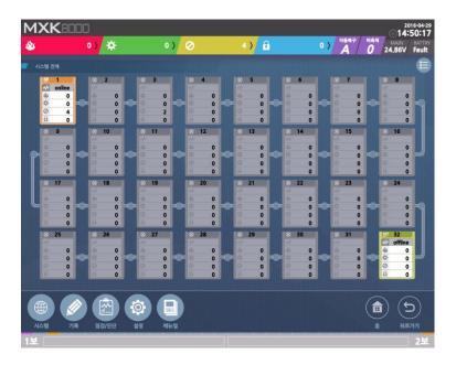
This screen appears when you select the **system menu**. It shows the status of each panel connected to the network, along with the number of events for each panel.
