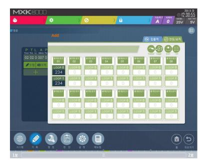
Touching the 'Inspection' button on the initial screen displays the screen above. Inspection is used to check the information about input/output circuits downloaded to the panel and identify any errors or problems. The screen above displays virtual inputs and outputs that do not operate in real-time.
