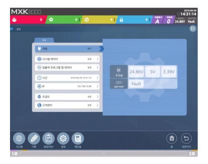
Touching the 'Power' button on the Setup screen displays the screen above.
