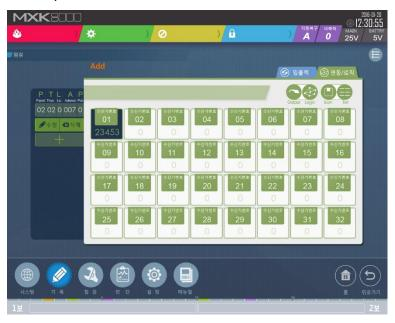
The selected input is displayed on the left side, and the corresponding output number is shown on the right side. Clicking the number displays the output information or the entire list, as shown below.
