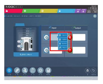
An inverted image in the Input or Output area indicates that the circuit is selected.
