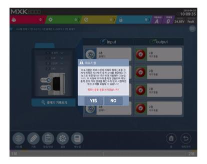
The screen above explains the hazards that may occur during the circuit test. The user must read this carefully before proceeding and pay special attention to the potential damage that could result from the test.
