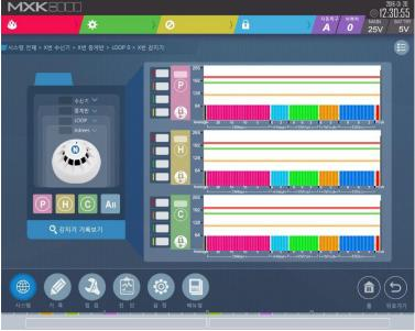
The screen above is about an analog type detector with two or three kinds of information. Touch the red box on the screen to see the warning statement and isolate the circuit.
