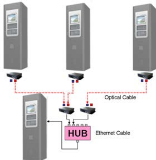
< Figure 6-15: 4 Panels, Optical Network Connections >
