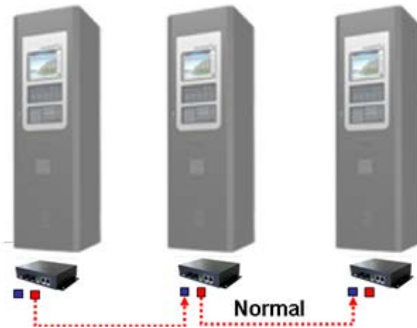
< Figure 6-16: 3 Panels, optical network connections (Bus) >
