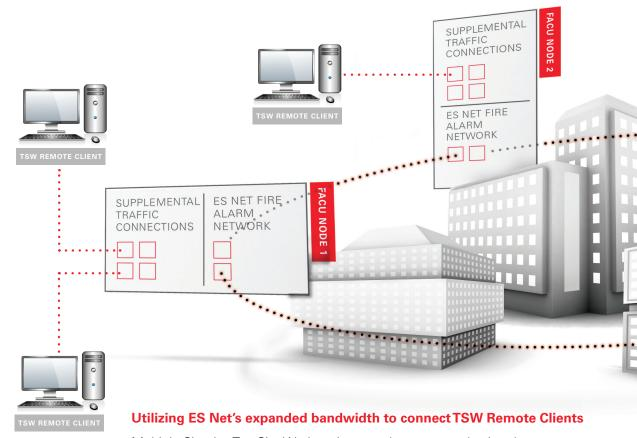
Multiple Simplex TrueSite Workstations can be connected using the supplemental traffic channel of ES Net, negating the need to set up a separate network. This results in significant savings of time, materials and resources without sacrificing network performance or reliability. The network can exist within a single building or across multiple buildings and works with a mix of network types (fiber, Ethernet, etc.).
