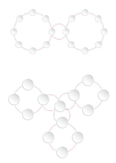
ES Net eases design and installation by supporting ring, star, bus and bridged ring network topologies. Because you can combine multiple topologies, you can create fault-tolerant, highly survivable networks while mixing and matching media between nodes to optimize cost, distances and performance.
